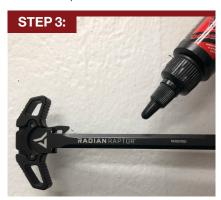
Place lubricant on the sides and top of the charging handle.
