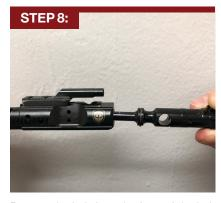
Remove the bolt from the front of the bolt carrier.
