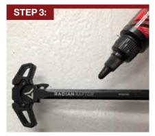
Place lubricant on the sides and top of the charging handle.
