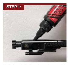
The bolt carrier body and campin, especially along the runners on the bottom of the carrier and the bosses on the rear, should be lubricated. Place two drops of lubrication into the campin slot.
