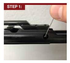
With a suitable punch or the tip of a cartridge, push the firing pin retainer in from the right-side, then pull it out from the left-side. Do not twist the retainer during removal.
