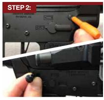
Make sure the bolt carrier group is in the forward seated position. From the left-hand side, press in the rear takedown pin. From the right-hand side, pull the rear takedown pin to the right until it stops.
