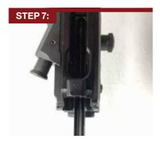
Pull the charging handle fully towards the rear. Remove the charging handle by moving it so that the expanded end of the charging handle passes through the cut-out in the guide track of the upper receiver.
