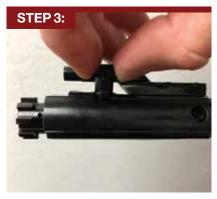
Rotate the cam pin to the side so that it is clear of the gas key. Lift the cam pin out of the bolt carrier group.
