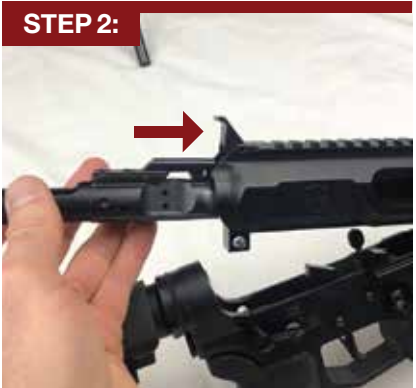
Ensure cover latch is lifted, slide bolt carrier into the upper receiver.
