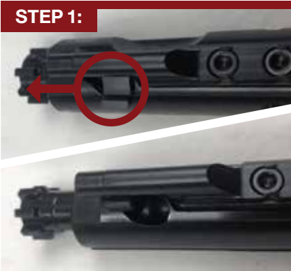
Make sure bolt and cam pin is all the way forward.
